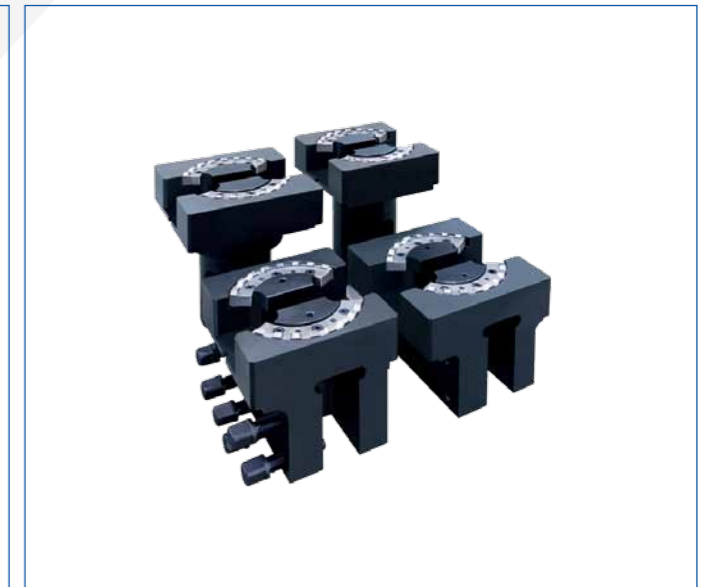
Tool holder: the thrusting cylinder installed on upper part of ram moves drag link up/down to forcefully raise and tightly pull tool holder, and lower fluted disc is used for positioning.
